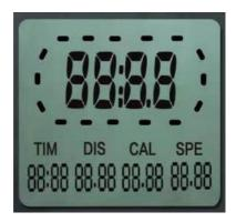
The main interface is used to display device name, time, distance, calories, speed,
